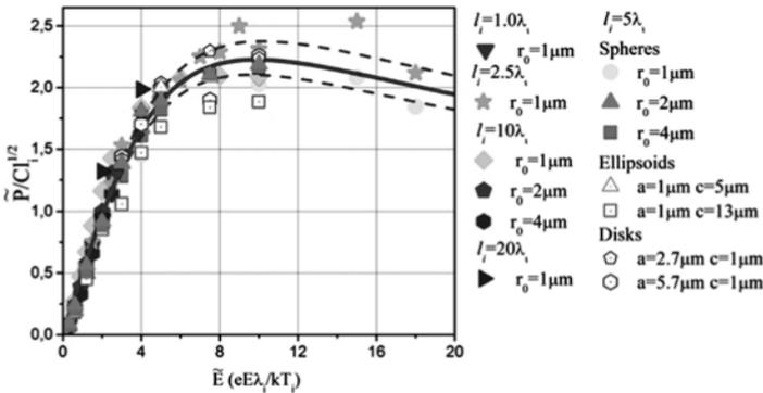
**Fig. 1.** A normalized dipole moment of an ion-electron cloud around a dust particle in an external electric field (C is the dust particle capacity,  $\lambda_i$  is the mean free path).
