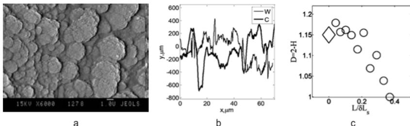
**Fig. 1.** (a) Micrograph of tungsten irradiated with high heat plasma [1]. Height profiles of tungsten (W) from the QSPA-T and the carbon (C) from the T-10 tokamak [1]. (c) Fractal dimension of equipotential lines (circles) vs a minimal distance  $L$  from the surface normalized by a maximal scale of surface irregularity  $\delta L_s$ . Diamond – fractal dimension of the real surface profile.
