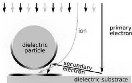
**Fig. 1.** The mechanism of charge accumulation and electrostatic lofting.
