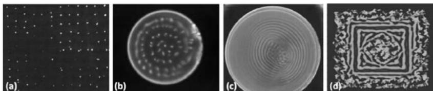
**Fig. 1.** Pattern formation in MDPX (viewed from the top): (a) dust particles, (b) single filaments, (c) filament rings, and (d) simulation of filaments.
