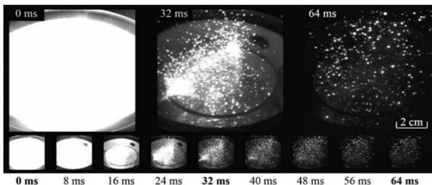
Fig. 1. Levitating particles over the regolith surface (time  $t=0$  ms corresponds to the end of the microwave pulse).
