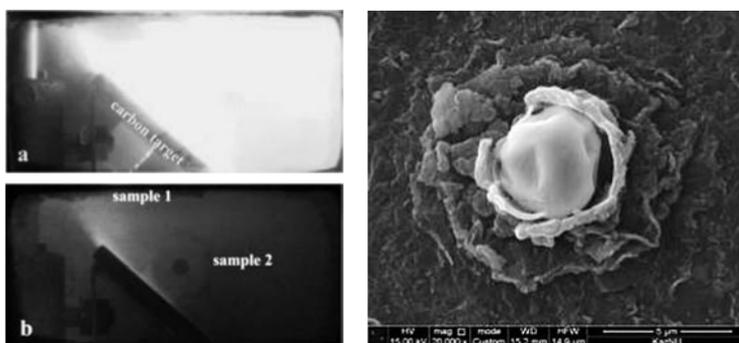
**Fig. 1.** Dust formation on the surface of a carbon target irradiated by a pulsed plasma stream
